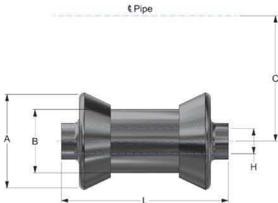
Fig. 501 Material: Cast Iron
