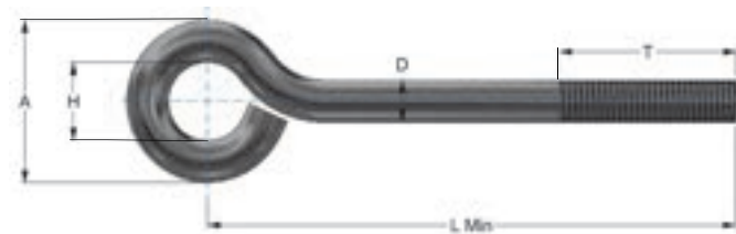
Fig. 3ER (Un-Welded) & 3ERW (Welded) – Eye Rod
