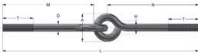
Fig. 3LE (Un-Welded) & 3LEW (Welded) – Linked Eye Rod
